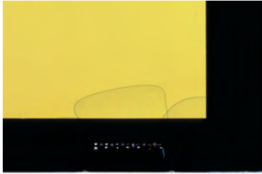
Fig. 7.14 This is a highly enlarged corner of a Drum-scanned 10x8 color transparency showing the clip mark and resultant bubbles in the oil. I had to twist someone's arm to capture this rare occurrence on film!
