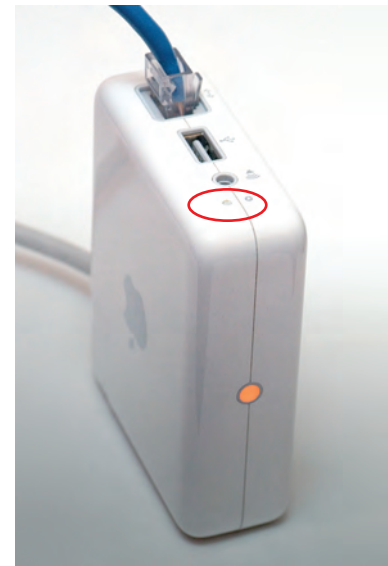
Fig. 7.34 The Reset button on the Airport Express Base Station often requires more than simply a press, and when used with the direct UK three-pin plug is difficult to access as the reset button lies on the underside of the unit.
