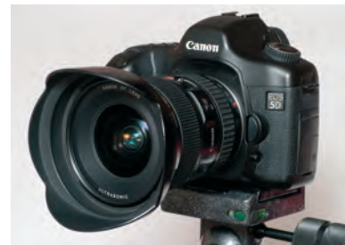
Fig. 7.19 Although not considered a fully professional camera, the Canon 5D is an excellent workhorse that is light enough to carry around for extended periods, takes the full range of lenses, has a large reviewing screen and has a 'full size' chip. So, for those used to 35 mm film SLRs, choosing a suitable lens for a particular angle of view, is second nature.
