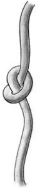
A SIMPLE OVERHAND KNOT CAN DE-RATE THE BREAKING STRENGTH OF A LINE BY AS MUCH AS 50%
